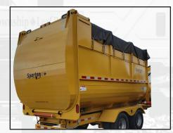
The Spartan Leaf Pro is a self-contained system designed to be pulled behind a towing vehicle. Benefits include being able to store more debris and stay out on the road for longer, with quick and easy emptying.
