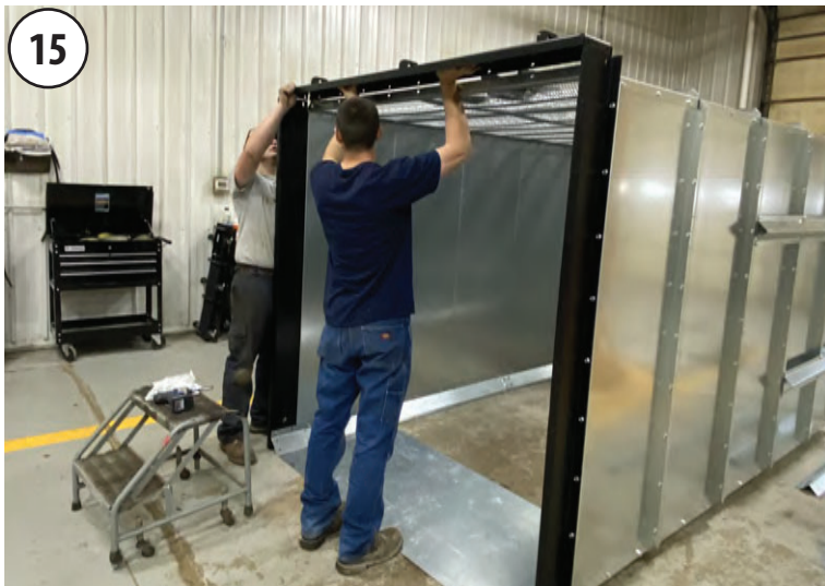
Bolt the tailgate hinge support to the tailgate support channels & top panel with (12) 5/16"-18 x 1" flange screws & 5/16"-18 locknuts.
