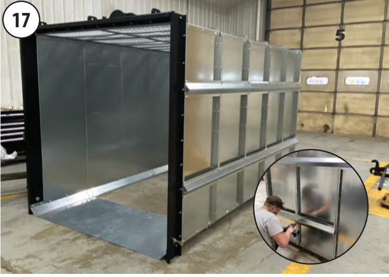
Install side reinforcements on the side panels with 5/16"-18 x 1" flange screws & 5/16"-18 locknuts. The short & long side reinforcements should be staggered for added strength.
