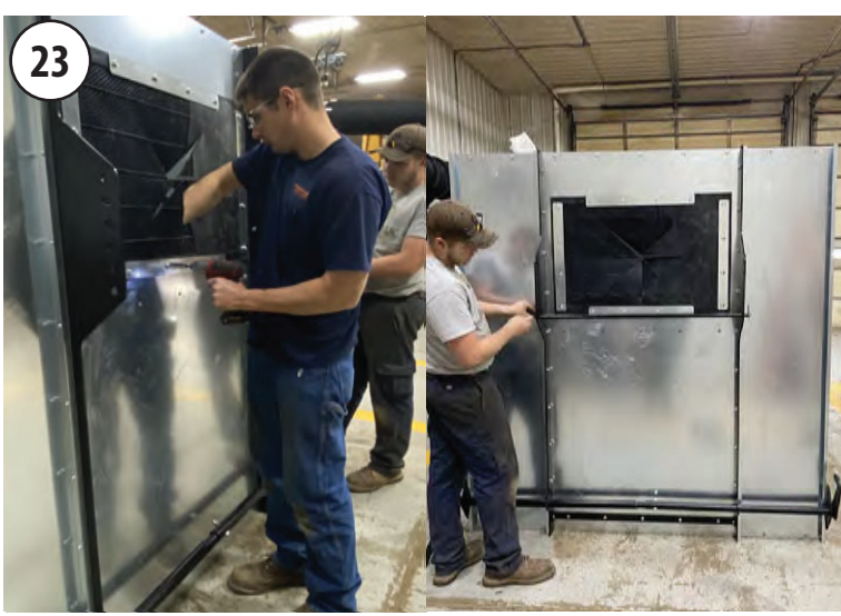
Assemble the rubber insert and (4) retainer strips with (16) 5/16"-18 x 1" flange screws & 5/16"-18 locknuts.
