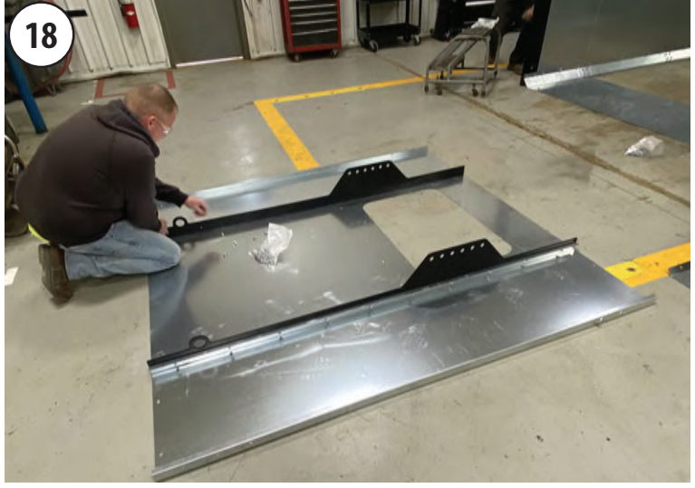
Assemble the tailgate by bolting (1) tailgate end panel & (1) rear vertical stiffener to each side of the tailgate center panel with (9) 5/16"-18 x 1" flange screws & 5/16"-18 locknuts.
