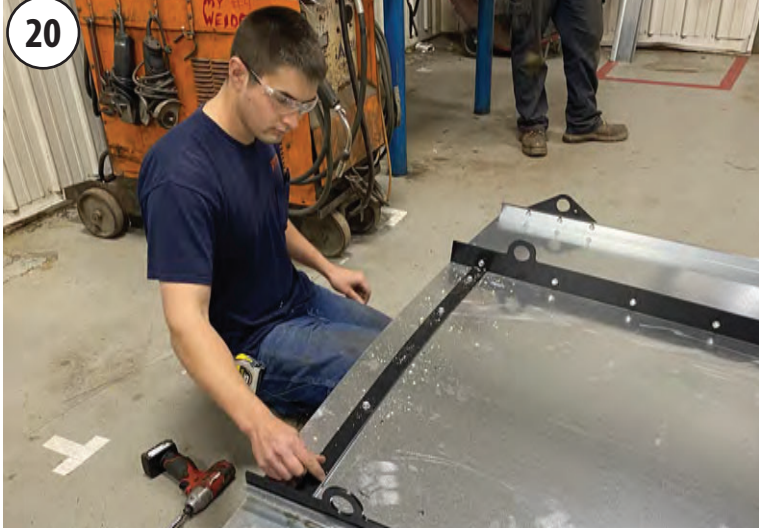
Bolt on the (2) tailgate center supports with (5) 5/16"-18 x 1" flange screws & 5/16"-18 locknuts each.
