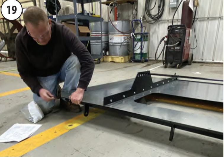
Bolt the tailgate hinge angle to the inside of the tailgate assembly with (9) 5/16"-18 x 1" flange screws & 5/16"-18 locknuts.
