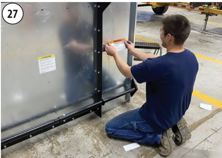
Apply the safety decals to the tailgate.
