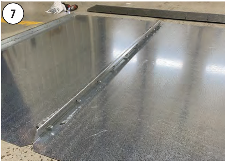
7 Bolt the side panels together with (9) 5/16"-18 x 1" flange screws & 5/16"-18 locknuts.
