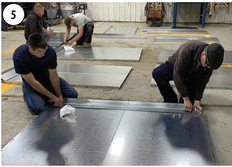
5 Bolt the front channel to the front panels with (8) 5/16"-18 x 1" flange screws and 5/16"-18 locknuts.
