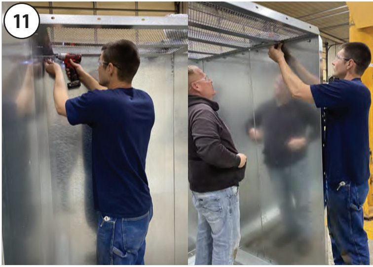
Install (2) top panels with (14) 5/16"-18 x 1" flange screws & 5/16"-18 locknuts each.
