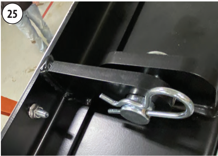
Assemble the tailgate assembly to the leaf box with (3) 1" x 2" clevis pins and hairpins.
