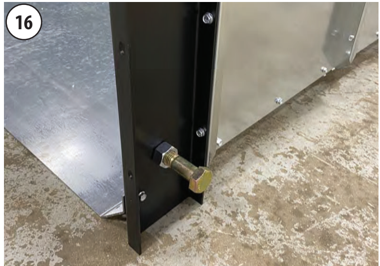
Assemble (1) 1"-8 x 4-1/2" bolt & (2) 1"-8 hex nuts to each tailgate support channel.
